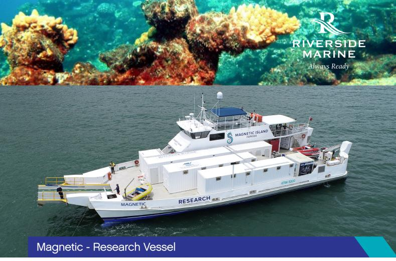
The vessel Magnetic has been transformed into a research vessel to provide a platform for marine biologists conducting research on the Great Barrier Reef. The large open areas available on board (420m2), allows for a variety of specialised modules to be craned on and off the vessel as per the research requirements. This approach gives scientists flexibility based on their research requirements. The vessel can accommodate 16 people (including 4 crew) for overnight stays with full catering.
